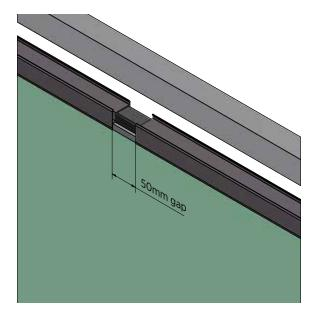
A gap of 50mm is needed to avoid LED and Handrail damage due to elongation and contraction from heat related matters.
