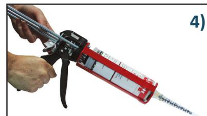
**PLEASE NOTE: ChemFix sets quickly.** Once you have applied it to the first 9-12 holes, twist the studding into each hole. Remove any excess ChemFix before it sets. Repeat this procedure until all holes are filled and leave to set for 60 minutes. Remember to change the Applicator nozzle.
